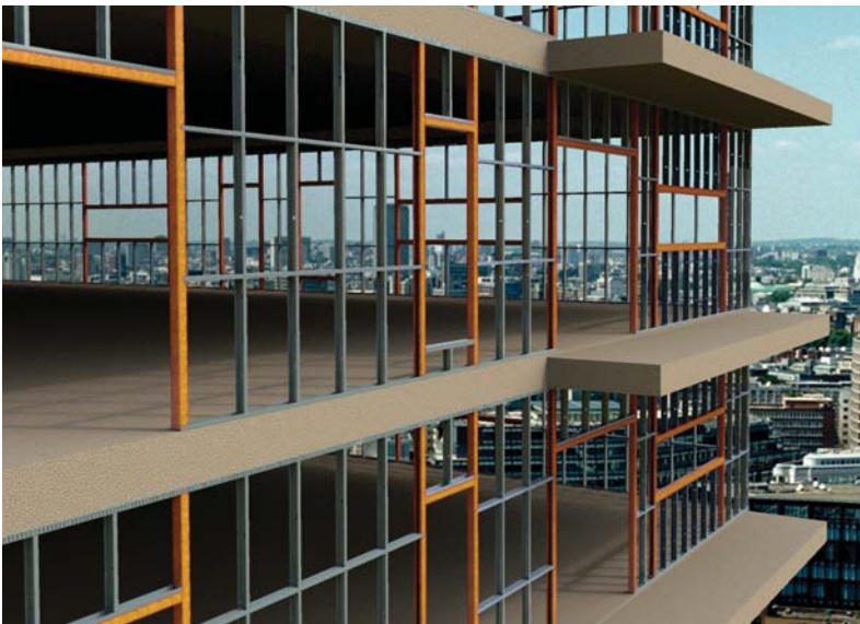
The HEDA System being used for all opening in steel stud construction
